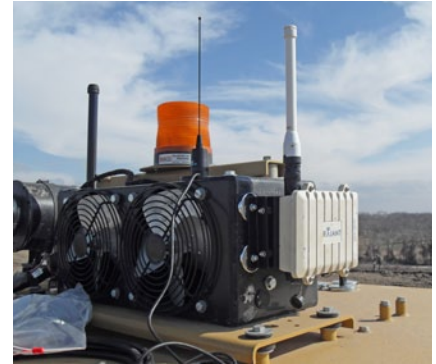
Network Radio—also mounted using high strength magnetic mount
