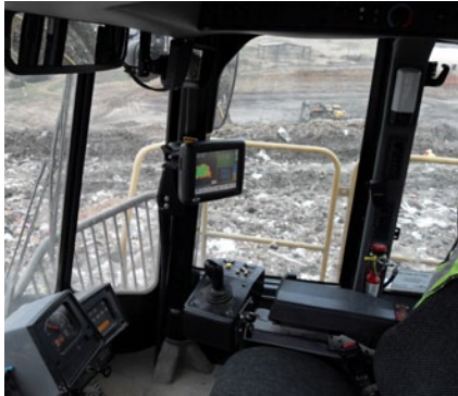
Computer / Display—mounted to the right within Reach of the operator
